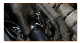
37 Screw in the fastener of the air intake pipe. Use Torx T25.
