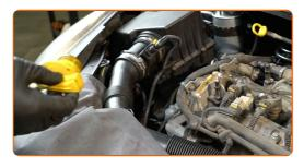
Tighten the oil filler cap.
