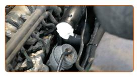
Undo the screws of the protective case of the oil filter housing. Use Torx T25. Use a drive socket #10. Use a ratchet wrench.
