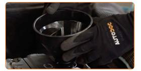
Pour new oil into the engine in the amount recommended by the car manufacturer.
