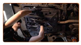
Tighten the fasteners of the oil pan lower cover. Use a drive socket #12. Use a ratchet wrench.
