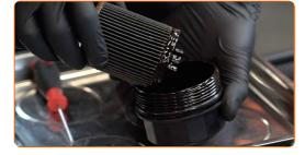
Remove the oil filter cover O-ring. Use a flat screwdriver. 17
