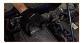
Fasten the clamp on the air intake hose. Use a drive socket #7. Use a ratchet wrench.
