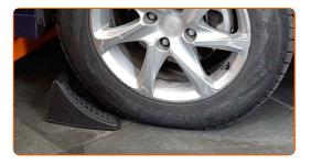
Loosen the wheel mounting bolts. Use wheel impact socket #17.
