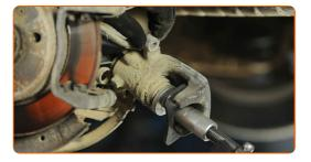
Install the brake caliper and fix it.
