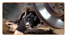
Tighten the fastener connecting the stabilizer link to the stabilizer bar. Use a combination spanner #17. Use a drive socket #19. Use a torque wrench. Tighten it to 60 Nm torque.
