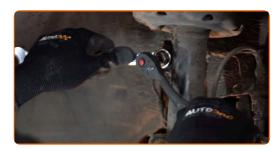
Unscrew the fastener connecting the stabilizer link to the shock strut. Use a combination spanner #18. Use a drive socket #8. Use a ratchet wrench.
