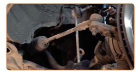
Replacement: anti roll bar links – OPEL Combo C Box Body / Estate. Tip from AUTODOC experts:
