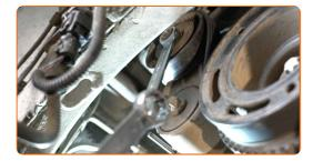
Place the serpentine belt on the crankshaft pulley.
