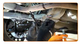
Cut the thread for the new oxygen sensor. Use a thread tap. Use a ratchet wrench.
