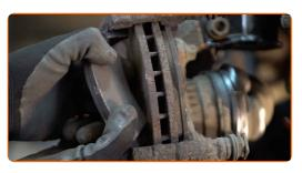
Replacement: brake pads – OPEL COMBO Box Body / Estate. Tip from AUTODOC:
