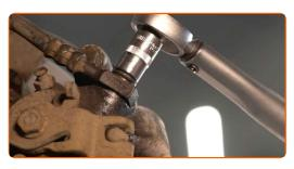
Remove the brake hose clamp.
