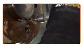
Remove the brake disc.
