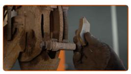
Clean the brake caliper bracket fasteners. Use a wire brush. Use a brake cleaner.
