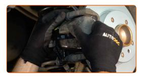
Tighten the brake caliper fasteners. Use a combination spanner #17. Use a drive socket #13. Use a torque wrench. Tighten it to 25 Nm torque.
