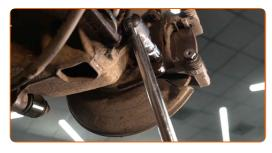
18 Remove the caliper bracket.
