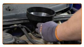
Pour coolant in the coolant reservoir.
