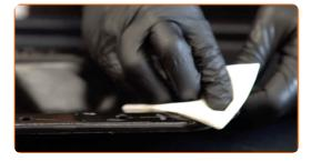
Apply sealant to the mounting seat of the transmission fluid pan gasket. Install the new transmission fluid pan gasket.
