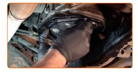
Tighten the fastening bolts of the transmission fluid pan in a criss-cross pattern. Use a drive socket #11. Use a torque wrench. Tighten it to 20 Nm torque.
