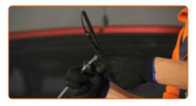
Remove the blade from the wiper arm.
