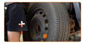
Remove the hub bearing protection cap. Use a flat screwdriver.
