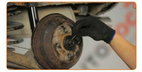
25 Install the hub bearing protection cap. Use a rubber mallet.
