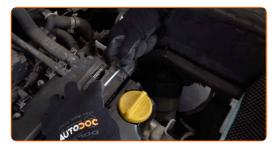
4 Unscrew the ignition coil bracket. Use Torx T30. Use a ratchet wrench.
