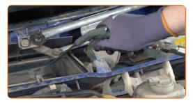
Insert a new filter element into the filter housing.
