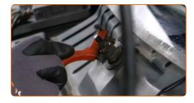
Unscrew the plastic panel fasteners. Use a combination spanner #24.
