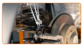
Unscrew the brake hose from the brake caliper. Use a combination spanner #11.
