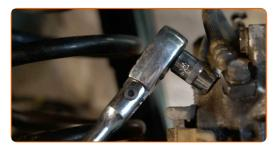
Connect the brake bleeder kit to the brake bleeder screw.
