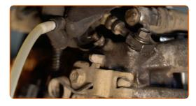
Tighten the brake bleeder screw. Use a drive socket #11. Use a ratchet wrench.
