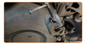
Install the brake caliper and fix it.
