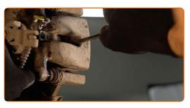
Remove the brake caliper. Use a crowbar.
