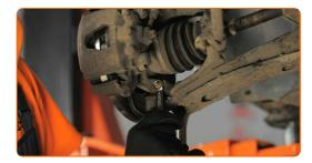
Remove the fastening bolt. Use a hammer.
