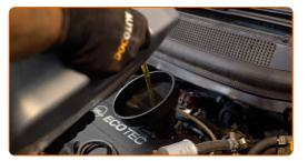
Replacement: engine oil and filter – OPEL Cascada (W13). AUTODOC recommends:
