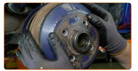
Replacement: wheel bearing - OPEL Calibra A (C89). Tip from AUTODOC:
