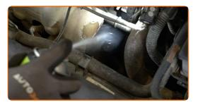
Unscrew the filter housing cap together with the old filter element. Use a drive socket #24. Use a ratchet wrench.
