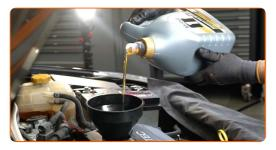
Replacement: engine oil and filter – OPEL Astra K Hatchback (B16). AUTODOC experts recommend:
