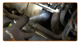
Unscrew the filter housing cap together with the old filter element. Use a drive socket #24. Use a ratchet wrench.
