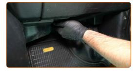
Screw in the fasteners of the bottom trim panel. Use Torx T20.
