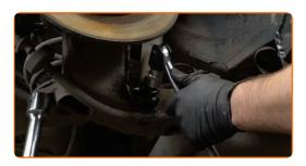
9 Remove the fastening bolt.
