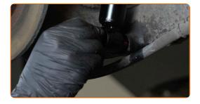
Screw in the lower fastener of the shock absorber. Use a drive socket #E20. Use a ratchet wrench.
