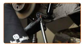
Tighten the top shock absorber fastening. Use a drive socket #18. Use a torque wrench. Tighten it to 90 Nm torque.
