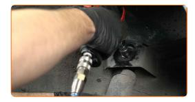
11 Remove the fastening bolt.
