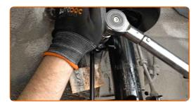
Tighten the fastener connecting the stabilizer link to the stabilizer bar. Use a drive socket #18. Use a torque wrench. Tighten it to 60 Nm torque.
