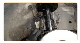
Tighten the stabiliser link fastener. Use a combination spanner #18.
