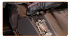
7 Unscrew the fasteners of the passenger side kick panel.
