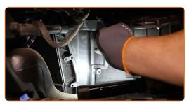
Screw in the fasteners of the cabin filter housing cover. Use a drive socket #5.5. Use a ratchet wrench.
