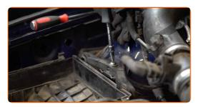
Insert the filter cartridge into the filter housing. Make sure that the filter edge fits tight to the housing.
