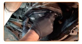
Tighten the fastening bolts of the transmission fluid pan in a criss-cross pattern. Use a drive socket #11. Use a torque wrench. Tighten it to 20 Nm torque.
