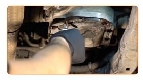
10 Remove the transmission fluid pan.
