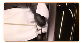
6 Attach the mirror heating connectors.
