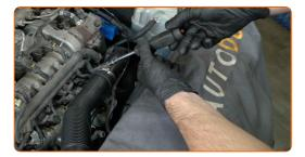
Disconnect the air intake pipe fastening. Use Torx T25. Use a ratchet wrench.
