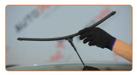
Remove the blade from the wiper arm.
