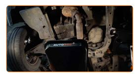
Clean the area of the oil pan drainage hole. Use a wire brush. Use all-purpose cleaning spray.
