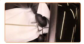
6 Attach the mirror heating connectors.
