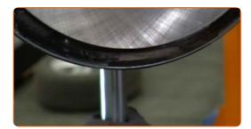
Tighten the lower fastener of the shock absorber. Use a drive socket #E20. Use a torque wrench. Tighten it to 130 Nm torque.
