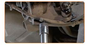
Unscrew the lower fastener of the shock absorber. Use a drive socket #E20. Use a tap wrench. Use a ratchet wrench.
