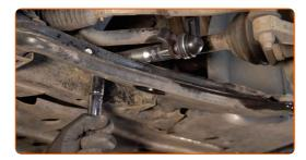
Tighten the fastener connecting the stabilizer link to the shock strut. Use a drive socket #19. Use a torque wrench. Tighten it to 55 Nm torque.
