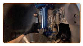
Tighten the fastener connecting the stabilizer link to the stabilizer bar. Use a drive socket #19. Use a torque wrench. Tighten it to 55 Nm torque.
