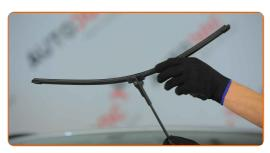
Remove the blade from the wiper arm.
