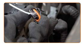
Replacement: spark plugs - OPEL Astra H GTC (A04). Tip:
