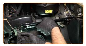
Screw in the fasteners of the air distribution housing assembly. Use a drive socket #10.
