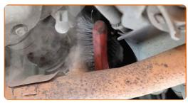
Detach the oxygen sensor connector.
