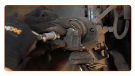
Clean the brake caliper bracket from dirt and dust. Use a wire brush.
