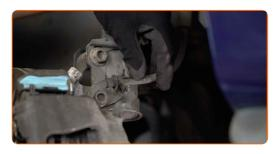
Install the brake hose retaining clip. Use a crowbar.
