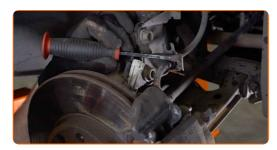
Pull aside the brake caliper retaining spring. Use a crowbar.
