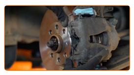
Fasten the brake hose on the strut.
