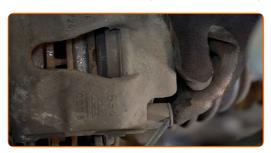
Unscrew the brake caliper fastening. Use HEX No.H7. Use a ratchet wrench.
