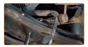
Unscrew the fastener connecting the stabilizer link to the shock strut. Use a combination spanner #19. Use a drive socket #19. Use a ratchet wrench.
