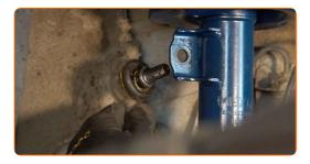
Replacement: anti roll bar links - OPEL Astra H GTC (A04). Tip:
