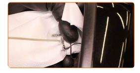
6 Attach the mirror heating connectors.
