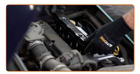
Tighten the ignition coil fastening. Use Torx T30. Use a torque wrench. Tighten it to 15 nm torque.
