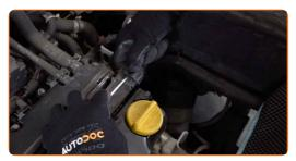
Unscrew the ignition coil bracket. Use Torx T30. Use a ratchet wrench.
