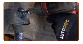
11 Remove the fastening bolt.
