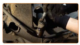
Unscrew the upper fastener of the shock absorber. Use a drive socket #E18. Use a tap wrench.
