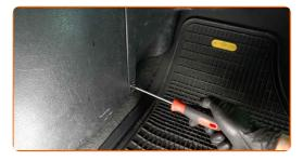
Remove the clips of the bottom trim panel. Use a clip removal tool.
