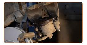
Replacement: brake pads – OPEL ASTRA H Box (L70). Tip:
