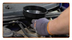
Pour coolant in the coolant reservoir.
