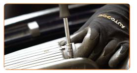
40 41 Remove the fender protection cover.
