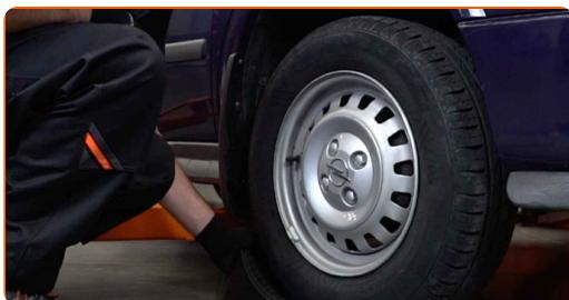
3 Loosen the wheel mounting bolts. Use wheel impact socket #17.
